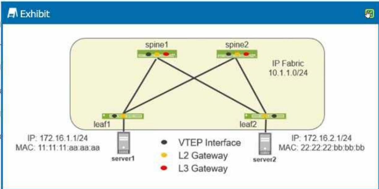
You have implemented an EVPN-VXLAN data center. Device served must be able to communicate with device server2.
